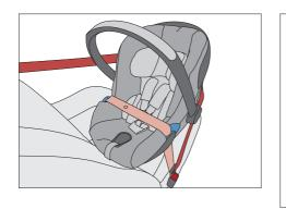
**【警告!** 即使不用时,也必须 用安全带将本婴儿安全座椅提篮 固定起来。如遇紧急刹车或事 故,未固定的婴儿安全座椅提篮 可能会伤到其他乘客或您自己。 **! WARNING!** The infant car seat must always be secured with the vehicle seatbelt, even when not being used. In the event of an emergency stop or a minor collision, an unsecured infant car seat can injure you and other passengers.
