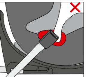
**!** **WARNING!** The vehicle belt buckle must never cross the belt guides. If the belt system is too long, the car seat is not suitable for use in this position in the vehicle. In case of doubt, please consult the manufacturer of your vehicle.
